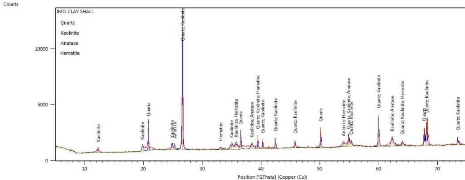
Fig.1. X-ray diffraction patterns of Urban Soils formed from Imo Clay Shale
