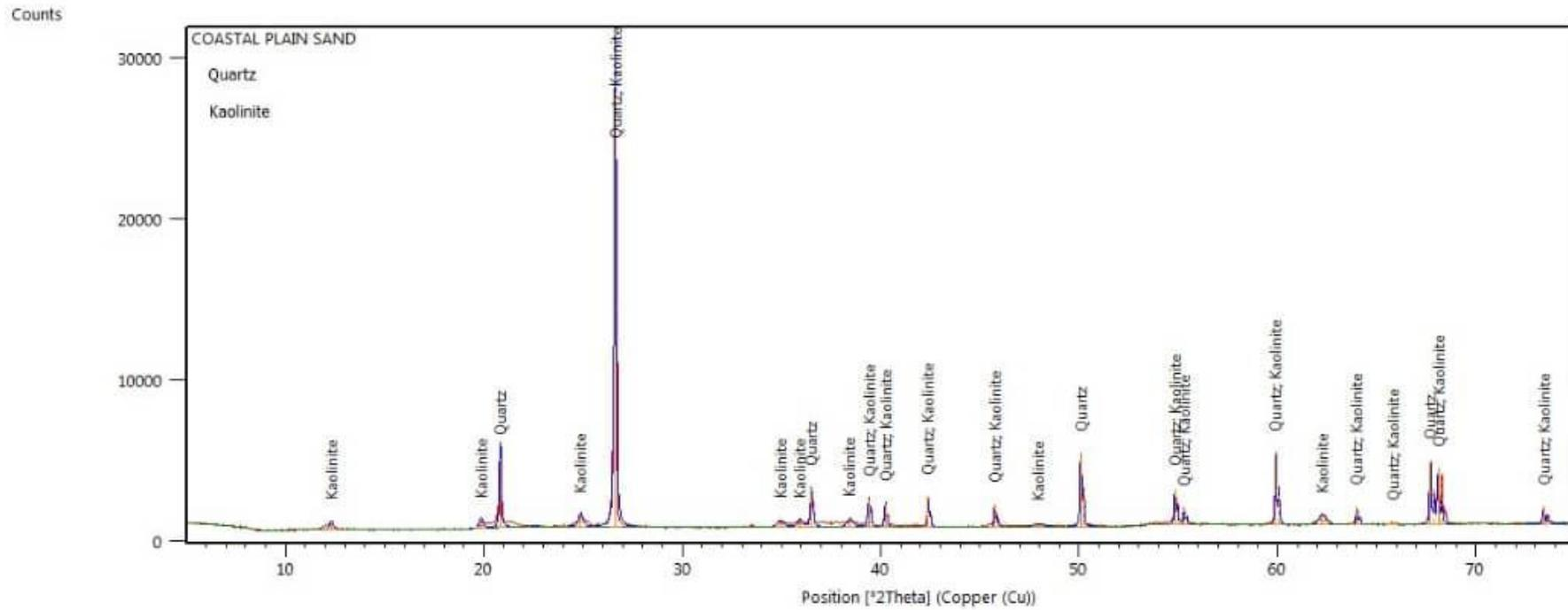
Fig.2. X-ray diffraction patterns of Urban Soils formed from Coastal Plain Sands
