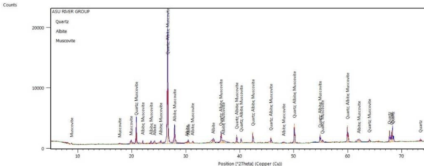
**Fig. 3. X-ray diffraction patterns of Urban Soils of Imo Clay Shale**
